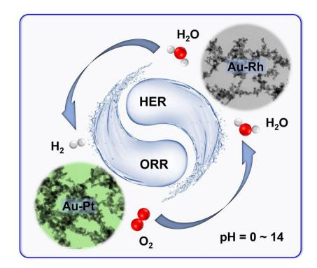
New-type noble metal aerogels were developed for outstanding pH-universal electrocatalysis toward hydrogen evolution reaction and oxygen reduction reaction. Credit: Wiley-VCH
