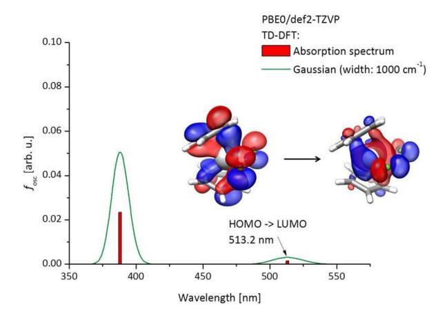
Calculated absorption spectrum of Titanocendichlorid [(C5H4)2TiCl2)] and molecular orbitals involved in the excitation. Credit: Tobias Hilche
