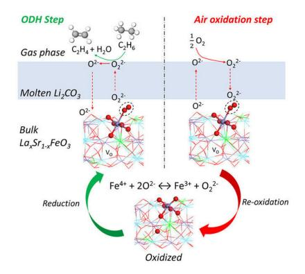
Reaction pathways for oxidative dehydrogenation of ethane facilitated by the molten carbonate shell modified perovskite redox catalyst. Credit: Fanxing Li, NC State University
