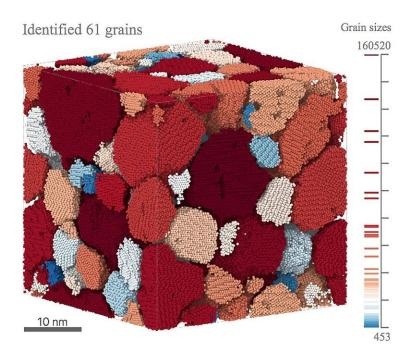
Machine-learning enabled characterization of 3D microstructure showing grains of different sizes and their boundaries. Credit: Argonne National Laboratory
