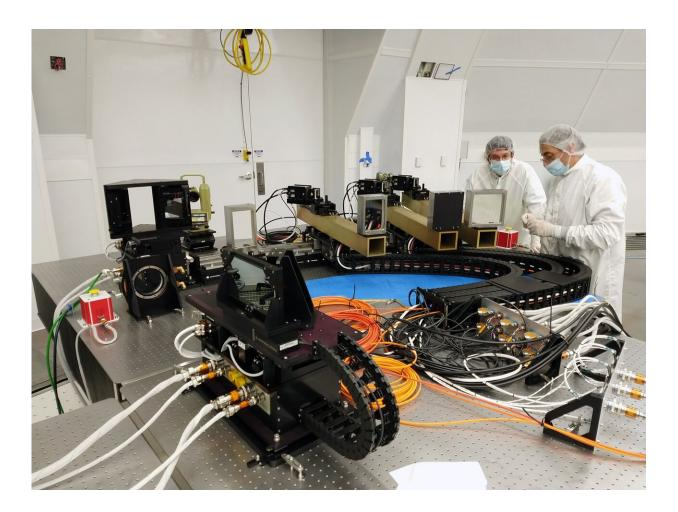
Predrag Sekulic of the National Solar Observatory (left) and Roberto Casini of NCAR's High Altitude Observatory (right) work on the three tunable spectral channels of the Visible Spectro-Polarimeter in the Inouye Solar Telescope's instrument room. Credit: Andrew Carlile, HAO
