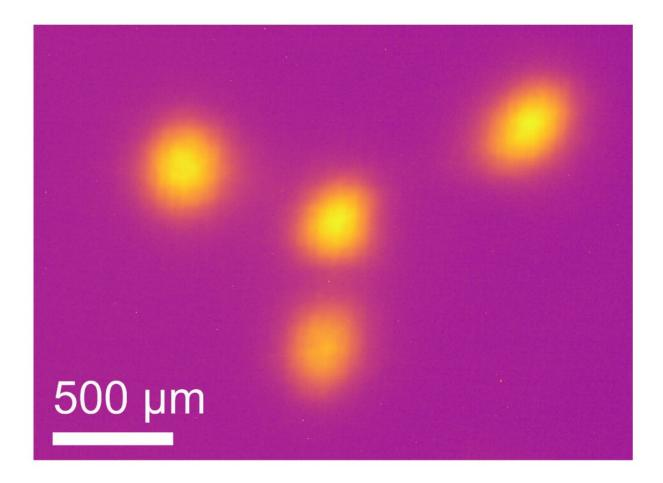
An X-ray image of the electron beam in TRIB-mode where two orbits co-exist: the regular orbit and the second one winding around it closing only after three revolutions. Credit: F. Armborst/K. Holldack/HZB
