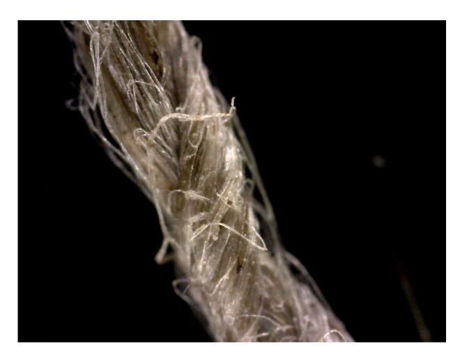
Close-up of modern flax cordage showing tisted fibre construction. Credit: S. Deryck
