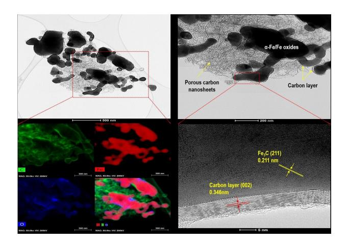
The KIST research team observed magnetic porous carbon composite materials in the transmission electron microscope. Researchers tested the efficiency of the porous carbon composite in terms of its ability to adsorb "tetracycline," or the antibiotic used to treat bacterial infections, from the water. Tests showed that the newly developed material was able to remove 100% of the tetracycline in about 90 minutes under general water conditions (pH 6), with an adsorption rate of
