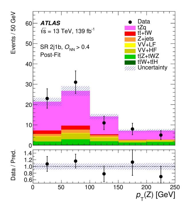
Figure 2: Distribution of the reconstructed Z boson transverse momentum for events with a neural network output (ONN) > 0.4. Data is shown in black. The simulated signal is shown in magenta. Backgrounds are shown in other colours. Credit: ATLAS Collaboration/CERN
