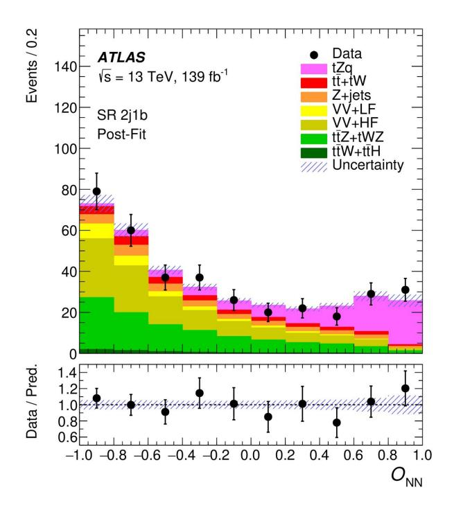
Figure 1: The neural network output (ONN) distribution for one of the signal regions. Data is shown in black. The simulated signal is shown in magenta. Backgrounds are shown in other colours. The high part of the ONN spectrum is dominated by signal events. Credit: ATLAS Collaboration/CERN
