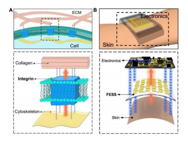
Bio-inspired in situ sensing and signal interconnection. (A) Conceptual illustration of the physiological information exchange between intracellular/extracellular matrices facilitated by cell adhesive molecules
