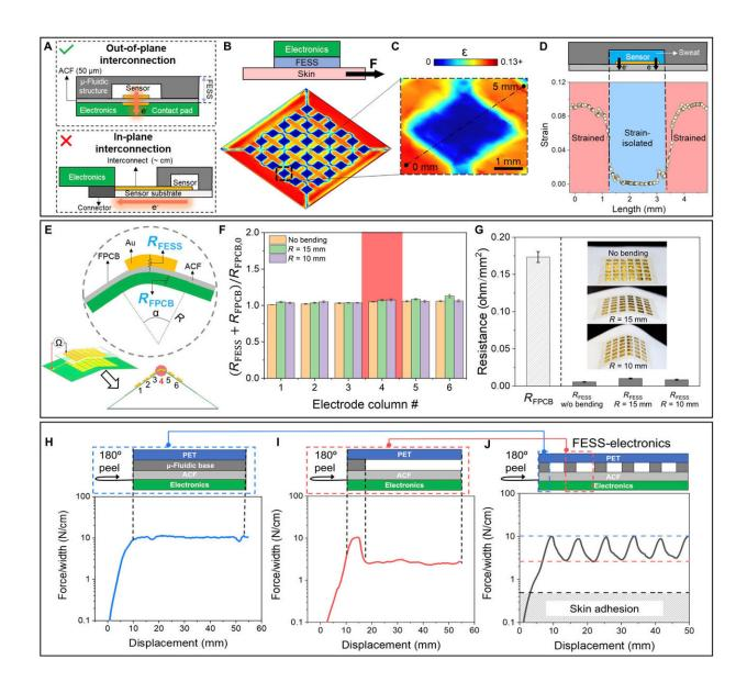
FESS strain simulation and characterization of strain-isolated signal interconnection. (A) Illustration of the FESS' out-of-plane signal interconnection versus conventional in-plane signal interconnection. Conventional implementations are constrained to signal routing through highly strained
