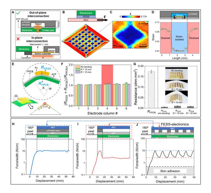
FESS strain simulation and characterization of strain-isolated signal interconnection. (A) Illustration of the FESS' out-of-plane signal interconnection versus conventional in-plane signal interconnection. Conventional implementations are constrained to signal routing through highly strained
