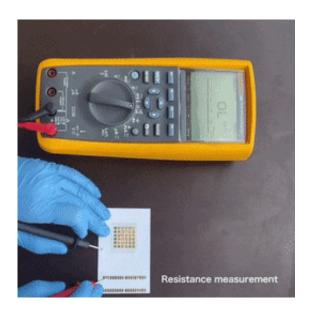
Testing the resistant measurement of the ACF-based interconnections after mechanical deformation. Credit: Science Advances, doi: 10.1126/sciadv.aaz0007
