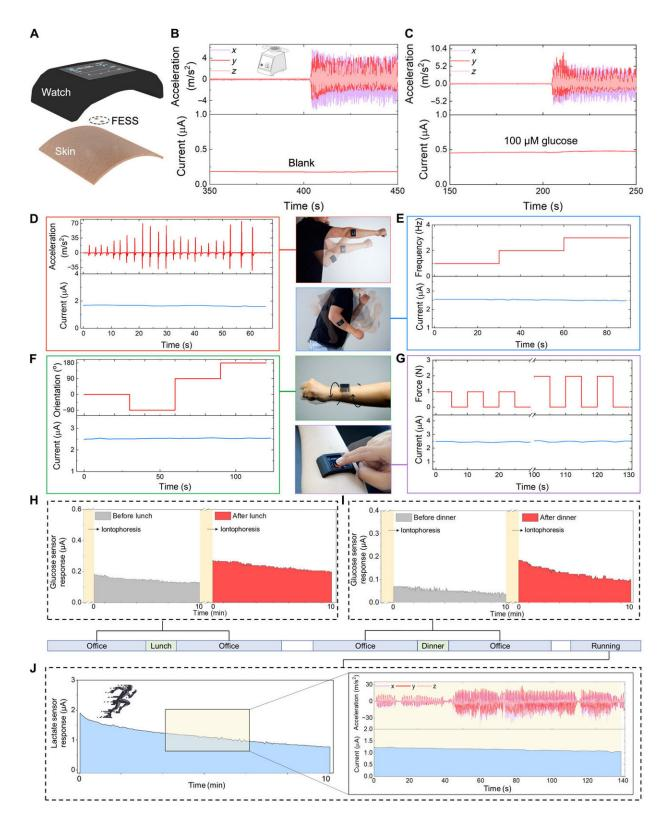
Custom-developed FESS-integrated smartwatch for on-body application. (A) Illustration of the FESS-enabled smartwatch (containing FESS, LCD screen,
