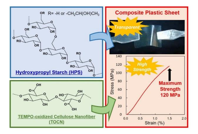
Fig. 2. Development of the transparent and high-strength starch/cellulose composite sheet. Credit: Osaka University
