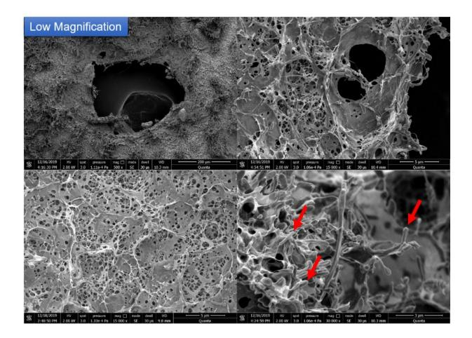
Fig. 3. Electron micrograph showing the marine biodegradability of the composite sheet. Credit: Osaka University
