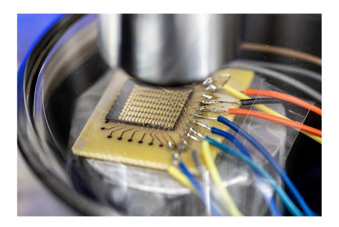
The pressure sensor the team designed operates over a wide range of pressures with high sensitivity. Credit: KAUST
