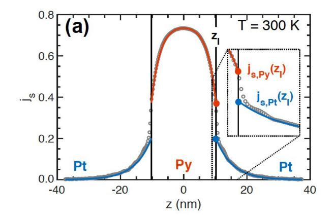
Open circles: spin current jS(z) through a Pt Py Pt trilayer calculated for T <sup>1</sup>/<sub>4</sub> 300 K. The solid blue (orange) curve is a fit to the VF equations in bulk Pt (Py). These fits are extrapolated to the interface zI to obtain the values js,Pt (ZI) and Js,Py (ZI)shown in detail in the right inset. (Left inset) The spin current with (red) and without (blue) proximity-induced moments in Pt. Credit: Gupta et al.
