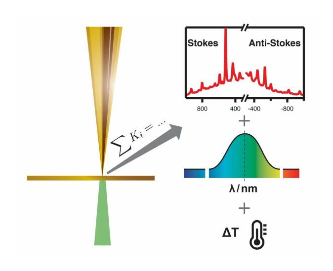
On the left side a schematic view of a tip-enhanced Raman scattering (TERS) experiment is shown. A metallized AFM probe is brought in close proximity to a specimen surface, a laser is focused on the tip-sample interface. Such a setup allows to obtain vibrational spectra (Raman spectra) of an extremely small region, as small as a single molecule or even a single bond. An example of so-
