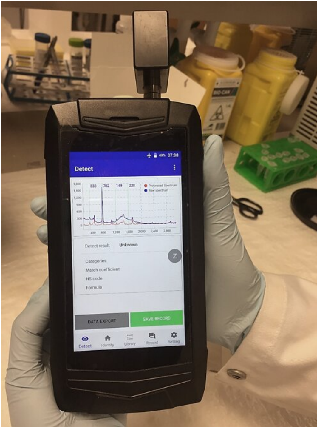
Non-invasive screening of cancer biomarkers from blood with handheld Raman reader. Credit: CNBP
