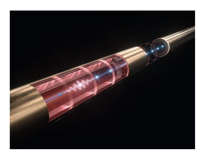
Proof of concept for cascaded terahertz accelerator using long pulses. The miniaccelerator uses terahertz radiation that can be recycled for a second stage of acceleration. Credit: DESY, Science Communication Lab
