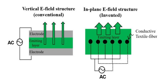
The structure of existing light-emitting device (left) and a new device with electrodes inside the light-emitting layer (right) Credit: DGIST
