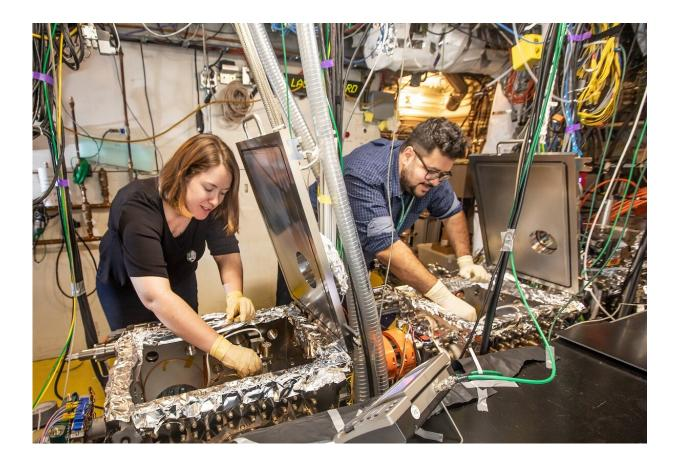
SLAC's Emma Snively and Mohamed Othman at the lab's high-speed "electron camera," an instrument for ultrafast electron diffraction (MeV-UED). Credit: Jacqueline Orrell/SLAC National Accelerator Laboratory
