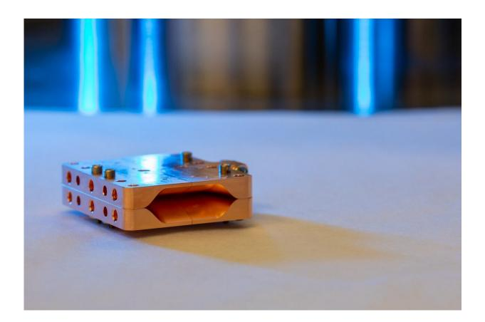
A compressor using terahertz radiation to shorten electron bunches is small enough to fit into the palm of a hand. Credit: Dawn Harmer/SLAC National Accelerator Laboratory
