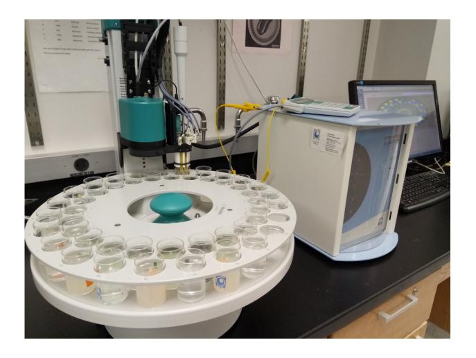
The researchers used WSU's e-tongue to measure the impact of reducing salt and the intensity of other ingredients with their new MATS processing technology. Credit: WSU
