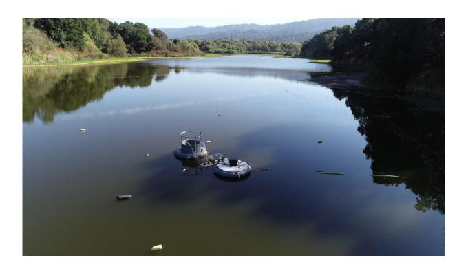
Downwelling field experiment at Searsville Reservoir in Woodside, California, which shows the pipes through which oxygenated surface water is pumped into the depths to prevent the formation of dangerous, low-oxygen dead zones. Credit: Nona Chiariello.
