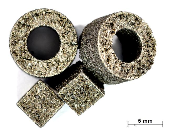
The research team has now succeeded in producing miniaturised supermagnets using laser-based 3D printing. Credit: IMAT – TU Graz
