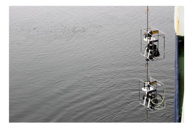
Algae samples from deeper water of the Arctic ocean layers were gained by using these in-situ-pumps. Credit: Max Planck Institute for Marine Microbiology/S. Becker
