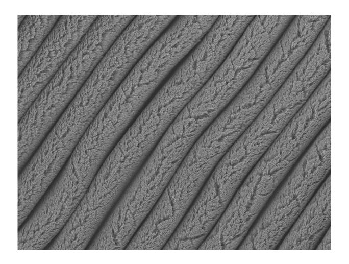
These forest-like rows of carbon nanotubes were created on an elastomer substrate that was pre-stretched in one direction and then allowed to contract. This process creates stretchable supercapacitors that hold more charge in less space and remain functional even when stretched to eight times their original size. Credit: Changyong Cao, Michigan State University
