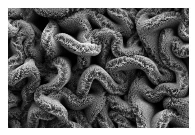
When carbon nanotube forests are placed on an elastomer substrate pre-stretched in two directions, it creates a maze of spaghetti instead of rows, improving the stretchable supercapacitor's performance. Credit: Changyong Cao, Michigan State University
