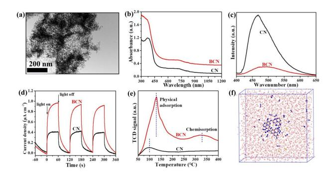
(a) TEM image of BCN; (b) UV-vis diffuse reflectance spectra, (c) steady-state PL spectra, (d) transient photocurrent responses and (e) N2-TPD of CN and BCN; (f) MD simulation snapshots of BCN. Credit: WANG Weikang
