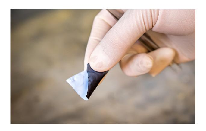
UC San Diego nanoengineers developed a separator that could make lithium metal batteries fail safely so that they do not rapidly overheat, catch fire or explode. Credit: David Baillot/UC San Diego Jacobs School of Engineering
