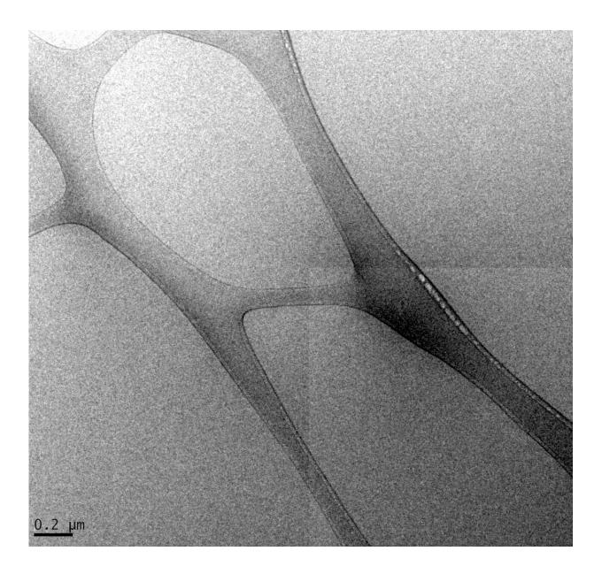
High-salinity brine mixed with crude oil does not appear to emulsify like low-salinity brine does, according to Rice University engineers studying the phenomenon. Their results have implications for enhanced oil recovery. Credit:
