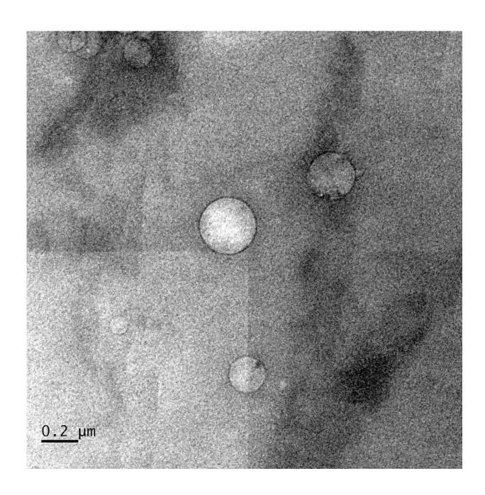
Low-salinity brine injected into crude oil forms nanoscale droplets that help
