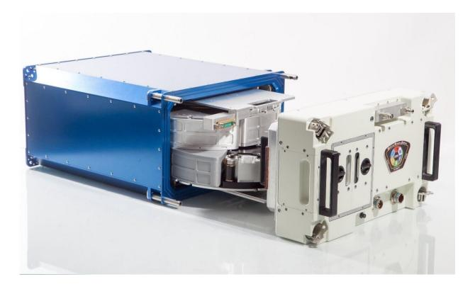
The Multi-use Variable-g Platform (MVP) used for the MVP Cell-03 experiment, shown with the MVP door removed and two carousels inside. Credit: Techshot, Inc.
