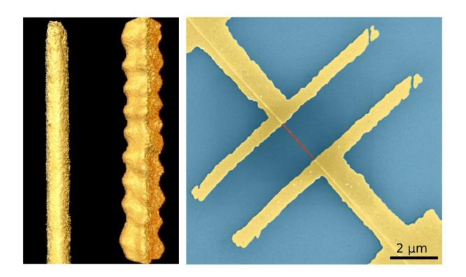
Left - Shape of nanostructures made of lead sulphide, computer reconstructed based on series of transmission electron microscopy images. The left straight stripe behaves like a semiconductor and the right zigzag nanowire behaves like a metal.Right - Electrical device consisting of two gold electrodes contacting a nanowire (in red) on a silicon chip (in blue). Credit: Hungria/Universidad de Cádiz, Ramin/DESY, Klinke/University of Rostock and Swansea University.
