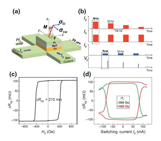
Measurement setup and type-z SOT switching. (a) Crossbar geometry with Ix, Iy ,  $\sigma$ sw, and  $\sigma$ bi inside. (b) Nonvolatile measurement sequence. Write and read processes are separated in the time domain. (c) Anomalous Hall resistance Rxy as a function of Hz. The maximum \_Rxy = 210 m\_. (d) SOT induced
