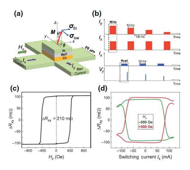
Measurement setup and type-z SOT switching. (a) Crossbar geometry with Ix, Iy ,  $\sigma$ sw, and  $\sigma$ bi inside. (b) Nonvolatile measurement sequence. Write and read processes are separated in the time domain. (c) Anomalous Hall resistance Rxy as a function of Hz . The maximum \_Rxy = 210 m\_. (d) SOTinduced
