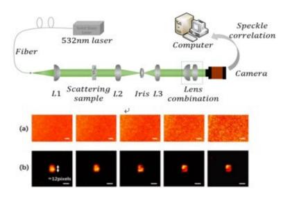
Experimental setup of speckle autocorrelation imaging with the 4f-configuration spatial filter and the results-the recorded speckle patterns and corresponding reconstruction images at different filter bandwidths. Credit: SIOM
