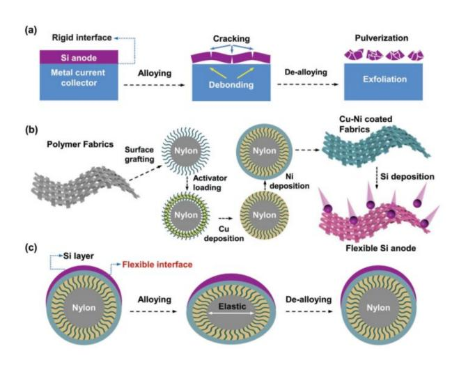
(a) Schematic illustration of the structural damage of silicon anode with a rigid interface design. (b) Fabrication process of silicon anode with fexible interface design on the soft nylon substrate with a Cu-Ni buffer layer. (c) The detailed structure of the fexible interface, and the shape change of the silicon anode during the alloying and de-alloying process. Credit: SIAT
