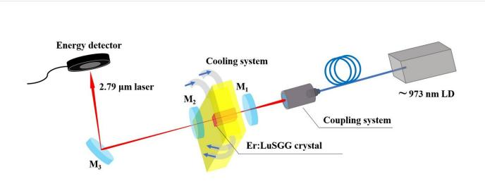
Schematic diagram of LD pumped Er:LuSGG laser. Credit: ZHAO Xuyao
