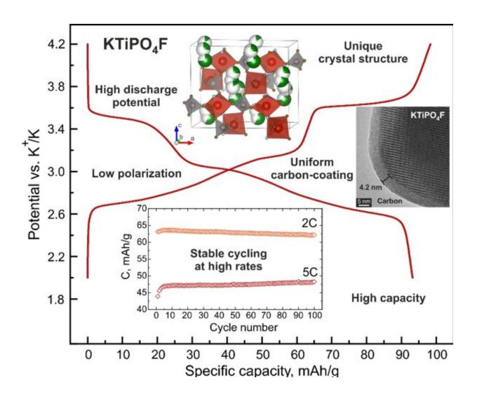
Researchers from the Skoltech Center for Energy Science and Technology (CEST) created a new cathode material based on titanium fluoride phosphate, which enabled achieving superior energy performance and stable operation at high discharge currents. Credit: Skoltech
