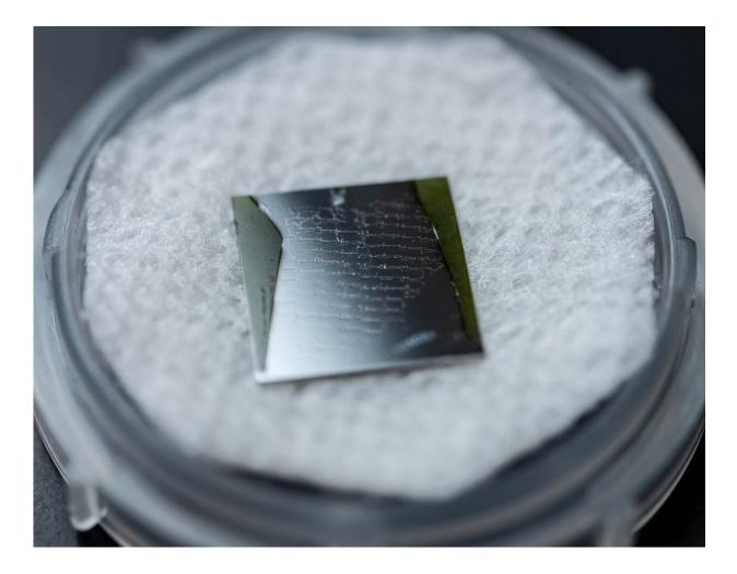
Closeup image shows polished GaN-SiC samples bonded by the surfaceactivated bonding technique. Credit: Rob Felt, Georgia Tech
