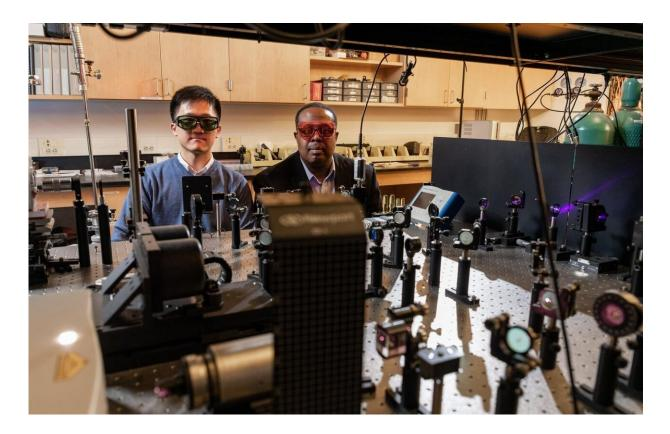
Researchers Cheng Zhe and Samuel Graham shown with an optical test setup for studying gallium nitride devices cooled by placement on a diamond substrate. Credit: Rob Felt, Georgia Tech
