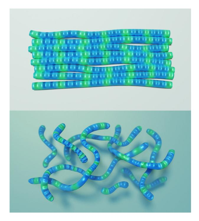
Solid vs. Liquid: Using gummy worms as a stand-in for the PCDTPT strands, these images depict the PCDTPT material in two forms: as a solid (top) and suspended in a liquid (bottom). In solid form, the gummy worms are touching, and electricity can flow from one worm to another. When suspended in a liquid, though, each gummy worm is more isolated, and electricity cannot flow as easily
