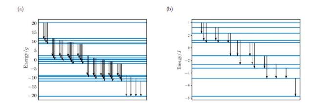
Possible paths via which an excitation can be cooled down to the ground state: Each black arrow corresponds to an energy difference  $\Delta - \gamma \le Ei - Ej \le \Delta + \gamma$ . Each cooling step leads to a reduction of the energy of the system, eventually reaching the ground state. The energy levels are shown for (a) the Ising model (N = 5, J/g = 5,  $\gamma$ /g = 3.5) and (b) the Heisenberg model (N = 5,  $\gamma$ /J = 1.26). Credit: Science Advances, doi: 10.1126/sciadv.aaw9268
