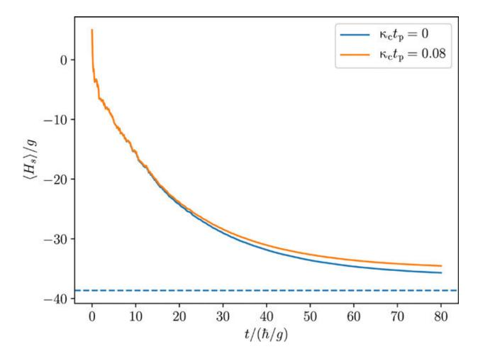
Cooling performance of an Ising-like chain of 5 + 1 ions of tp =  $80\hbar/g = 24$ s. The blue line shows the dynamics in the decoherence-free case resulting in a fidelity of f = 0.92, while the orange line indicates the dynamics under a collective decoherence mechanism with rate  $\kappa c = 3.3$ Hz, resulting in f = 0.89. The dashed line indicates the ground-state energy of the system. Credit: Science Advances, doi: 10.1126/sciadv.aaw9268
