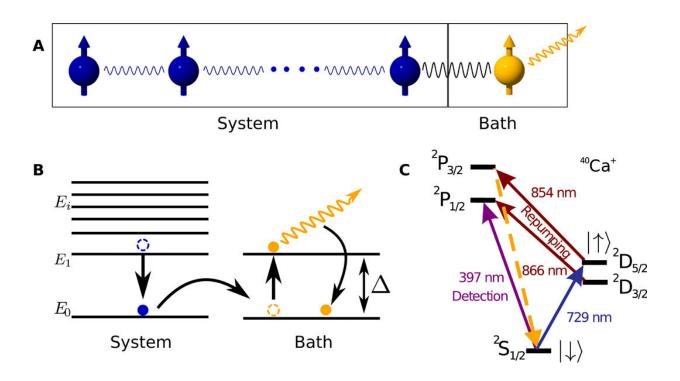
Sympathetic cooling of a quantum simulator. (A) A system of N spins performing the quantum simulation is interacting with an additional bath spin that is dissipatively driven. (B) Sketch of the energy level structure showing resonant energy transport between the system and the bath, after which the bath spin is dissipatively pumped into its ground state. (C) Level scheme for the implementation with trapped 40Ca+ ions. Credit: Science Advances, doi: 10.1126/sciadv.aaw9268
