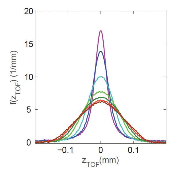
Evolution of the velocity distribution of a trapped gas of strongly interacting bosons expanding in one dimension. The initially peaked 'bosonic' distribution (purple line) gradually changes into the rounded 'fermionic' distribution (dark red line). The final shape is just like the Fermi sea that would characterize fermions in the same initial trap. Credit: Weiss Laboratory, Penn State
