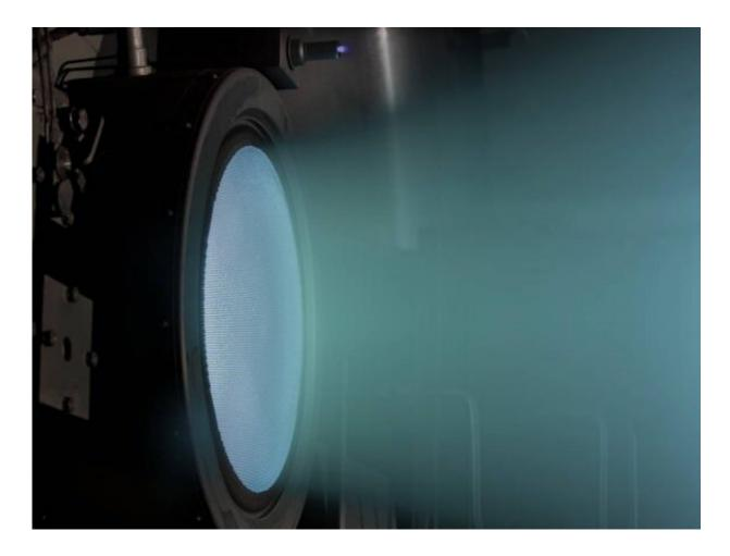
NASA Evolutionary Xenon Thruster being tested in a vacuum chamber. Credit: NASA
