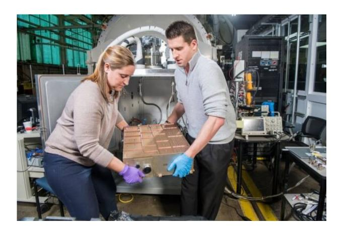
The power processing unit of the thruster is removed from another vacuum chamber after successful testing. Credit: NASA/Bridget Caswell
