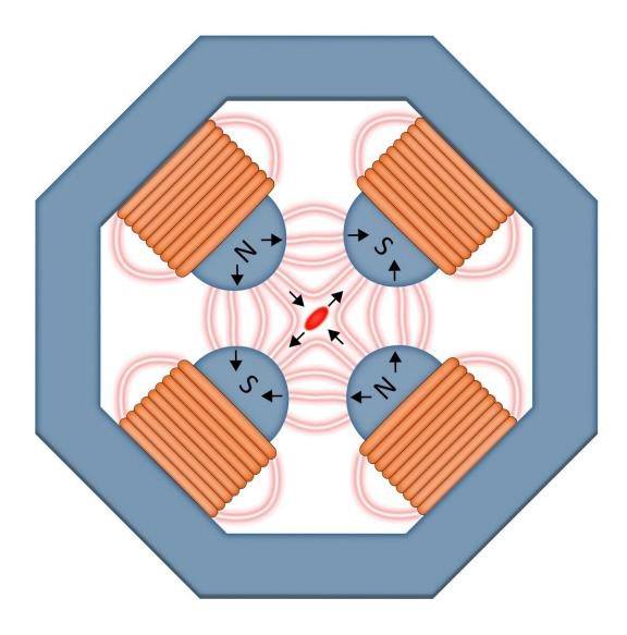
Quadrupoles have four magnetic poles. In a particle accelerator, the poles push particles together if they deviate too far from the centralized beam. Quadrupoles focus in only one plane, so to squeeze an accelerator beam from both sides, these magnets are usually stacked one after the other, each rotated by 90 degrees relative to the previous one. In this way, the beam particles are pushed together in both directions as they travel through successive magnets. Credit: Jerald Pinson
