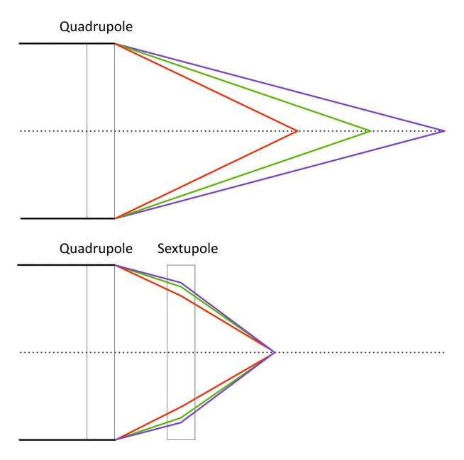
Quadrupole magnets are not able to focus particles with varying energies to a particular point, so scientists use sextupole magnets to correct for this chromatic aberration. Credit: Jerald Pinson
