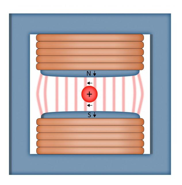
As a positively charged particle travels into the page and passes through the dipole magnet, it is deflected to the left at an angle proportional to the amount of force applied by the magnet. Credit: Jerald Pinson
