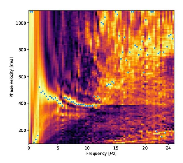
Analysis of seismic wave velocities using distributed acoustic sensing technique with fiber-optic cables. Credit: Zack Spica
