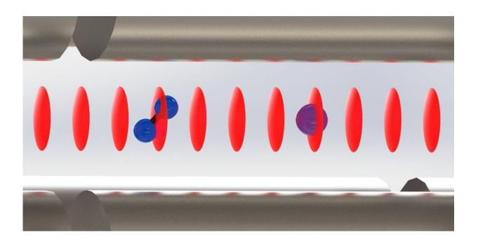
A charged nitrogen molecule is interrogated by a charged calcium atom in an optical lattice. Credit: University of Basel, Department of Chemistry
