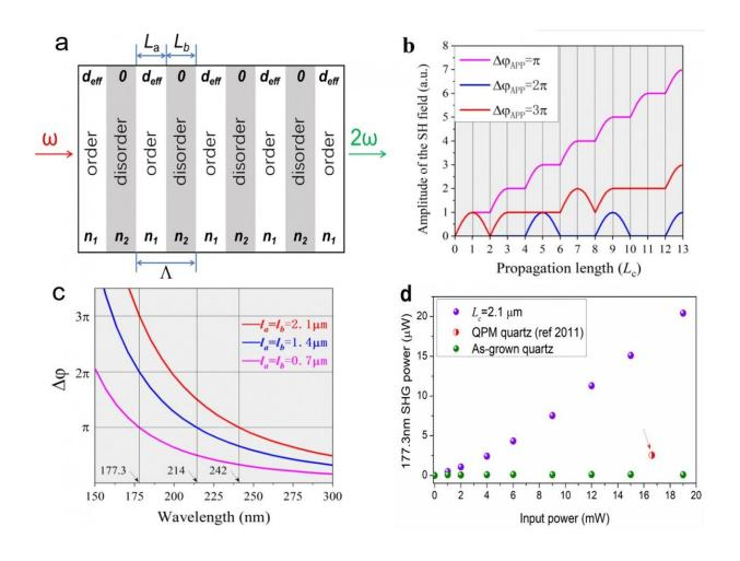
(a) Schematic graph of additional-phase-matching condition in arbitrary nonlinear optical crystals. The white and grey regions represent ordered crystal and disordered amorphous, respectively. The period length  $\Lambda$  equals the sum of ordered width La and disordered width Lb ( $\Lambda$  = La + Lb). Notably, La and Lb may be equivalent to coherent length Lc or integral multiple of Lc. deff/0 and n1/n2 represent the second-order nonlinear coefficient and refractive index of
