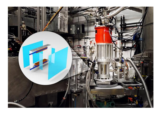
The spherical neutron polarimetry device features enhanced superconducting technology, coupled with an improved cooling system, adding new capabilities to US research by enabling the study of exotic magnetic phenomena in new dimensions. Credit: ORNL/Peter Jiang, Genevieve Martin
