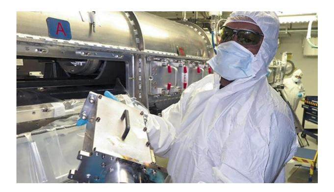
Target area operator Bill Board removes a neutron imager snout from a diagnostic instrument manipulator. The NIF neutron imaging system produces an image of the source distribution of the primary neutrons produced by fusion reactions and the lower energy neutrons that are downscattered in energy by the compressed fuel in an ICF capsule. Credit: Lawrence Livermore National Laboratory
