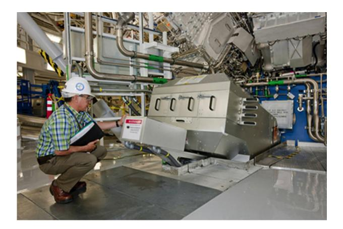
The magnetic recoil spectrometer (MRS) was developed by MIT and the University of Rochester's Laboratory for Laser Energetics to measure the neutron spectrum from an implosion by measuring proton (or deuteron) energy knocked out from a plastic foil held close to the implosion. MRS is a critical diagnostic for measuring the aerial density and yield of imploded targets, helping researchers quantify how well the shot is approaching ignition conditions. Credit: Lawrence Livermore National Laboratory
