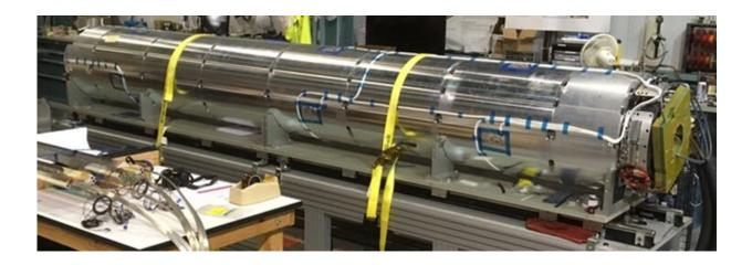
This new magnet reached the highest field strength ever recorded for an accelerator focusing magnet. Designed and built by Fermilab, Brookhaven National Laboratory and Lawrence Berkeley National Laboratory, it will be the first niobium-tin quadrupole magnet ever to operate in a particle accelerator — in this case, the future High-Luminosity Large Hadron Collider at CERN. Credit: Dan Cheng, Lawrence Berkeley National Laboratory
