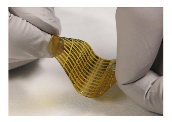
The nanoscale terahertz wave generator can be implemented on flexible substrates. Credit: EPFL / POWERlab
