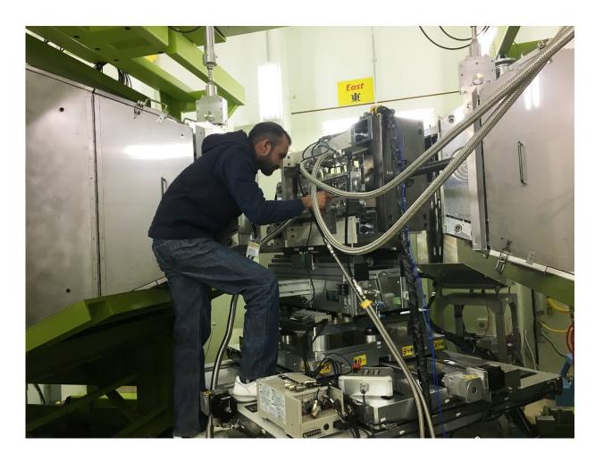
Muhammad Naeem prepares the experiment at TAKUMI, an engineering materials diffractometer at Japan Proton Accelerator Research Complex (J-PARC) used to perform in-situ neutron diffraction measurements multiple HEA samples, which all showed a multi-stage deformation process. Credit: © Professor Wang Xunli / City University of Hong Kongc
