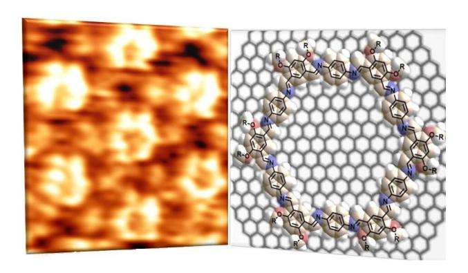
Experimental image of seven macrocycles on a graphite surface acquired through a Scanning Tunneling Microscope (Left) and a simulated macrocycle over a graphene surface (Right). Credit: Chaoying Fu
