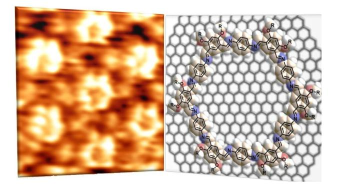
Experimental image of seven macrocycles on a graphite surface acquired through a Scanning Tunneling Microscope (Left) and a simulated macrocycle over a graphene surface (Right). Credit: Chaoying Fu
