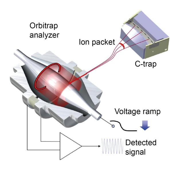
The Orbitrap. The ions that pass through it, circle around an electrode, producing an electric current signal. Credit: Utrecht University Faculty of Science
