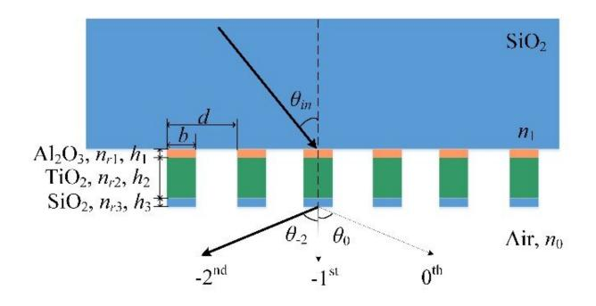
The schematic of high-efficiency three-layer transmission grating. Credit: SIOM
